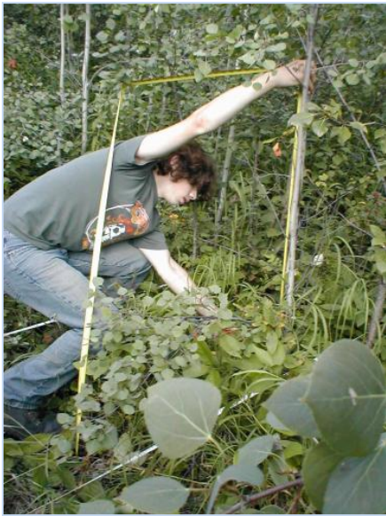
Nathan Stillwell measuring shrub biomass. This task is done in a 1-metre square area on each and every tree/shrub over 1 inch in diameter.
